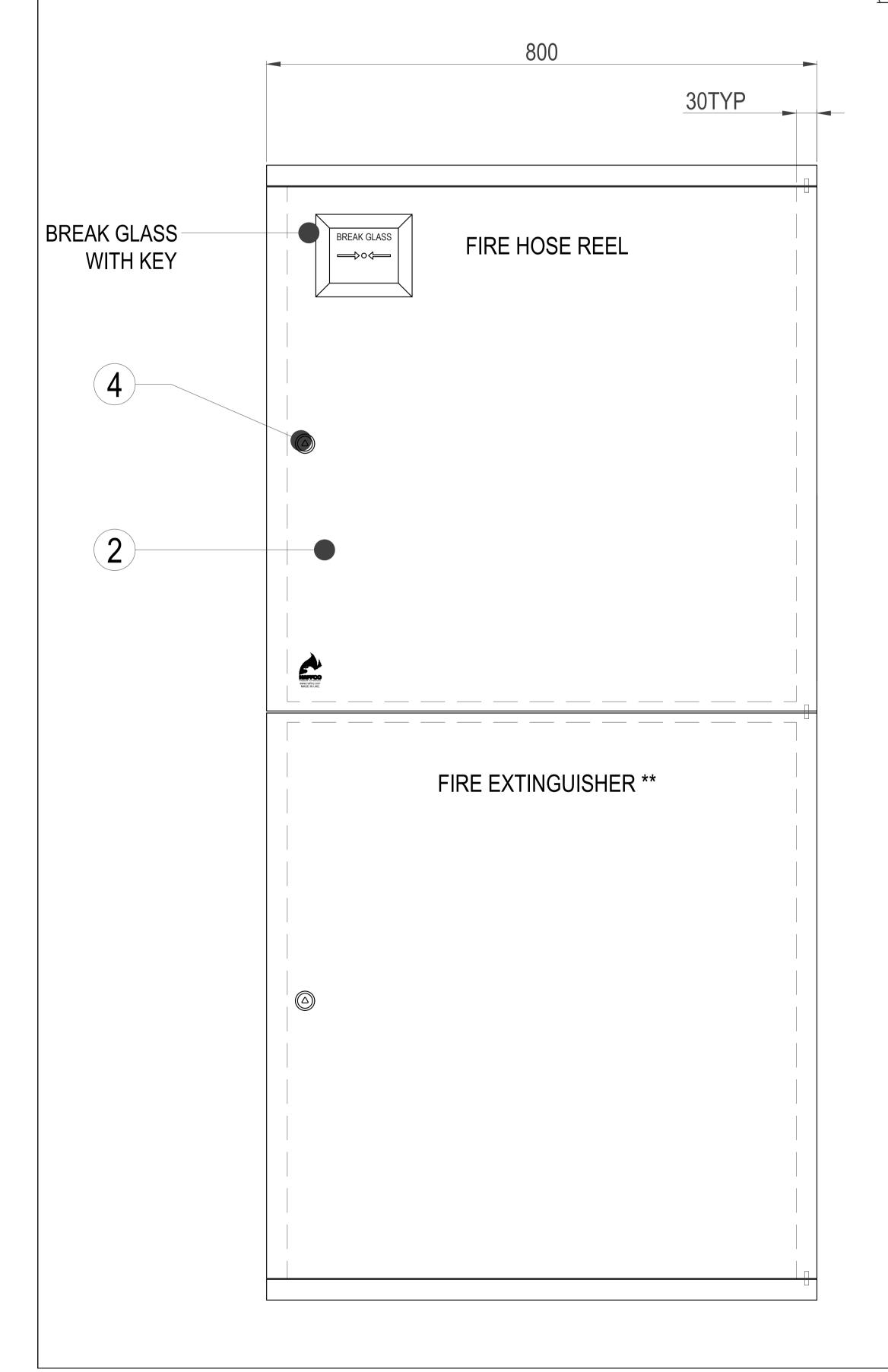
FIRE HOSE REEL CABINET DOUBLE VERTICAL SURFACE MOUNTED, COMPLETE STAINLESS STEEL BRUSH FINISH, WITH SOLID DOOR WITH BREAK GLASS AND KEY (MODEL: NF-SSBK-900)
